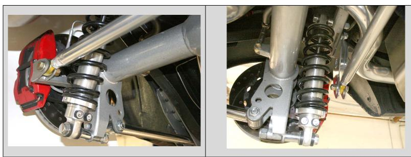
The photo on the left shows the panard bar attached to the axle housing bracket using  $\frac{1}{2} \ge 20 \ge 2$  inch bolt, washers and Nylock nut. The process is repeated on the right side on the panard bar bracket that is bolted to the coil-over cross-member. The three hole adjustment gives the choice of raising or lowering the rear roll center. Finish the project by installing the shock hole block off plates using the four  $5/16 \ge 18 \ge 34$  button head bolts.
