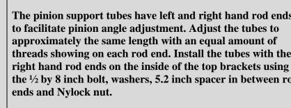
The left hand end of the tube is installed on the inside of the Torque Arm bracket with the spacer between the rod end and the Torque Arm tube. Install the ½ by 8 inch bolt through the bracket, rod ends, tube and spacers. Install Nylock nut and tighten. Now, tighten the nut on the bottom of the housing.
