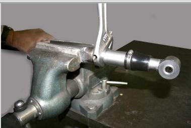
The Torque Arm is shipped with the slider assembly separate to facilitate packaging. The slider has preassembled with Teflon bushings and has been installed in th Torque Arm to check for proper fit. We use anti-seize on th threads to prevent galling. When painting or powder coatin the assembly, tape the threads on the slider and plug the ho in the Torque Arm tube.
