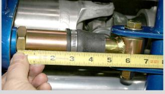
The slider shaft travels in and out very little but still needs be positioned in the slots 6<sup>1</sup>/<sub>4</sub> inches from the back of the wrench flats on the housing to the center of the sleeve with the bushing in it. This adjustment allows the slider shaft to be in the middle of its travel. Tighten the Nylock nut.
