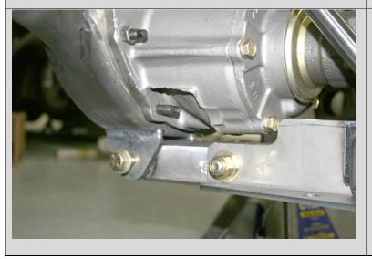
Install the rear of the Torque Arm to the tabs on the botton of the rear end housing using a ½ inch by 3½ inch bolt, washers and nut. Lightly tighten.
