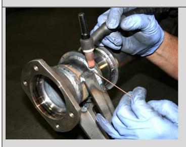
Finish welding the axle brackets and the panard bar brack as pictured. If an <u>optional</u> sway bar is being used the sway bar brackets are located on the front of the axle tubes at ax centerline on 33 inch centers.
