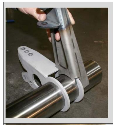
The axle brackets are designed to slide over a 3 inch axle tube before the bearing flange housings are installed. If the bearing ends are already on the axle bracket 3 inch ribs can be cut 90 degrees to the flat shock mounting face and reattached after the bracket is tacked on. The brackets are positioned 44 1/8 centers for stock width and 40 1/8 for the inch mini-tub.
