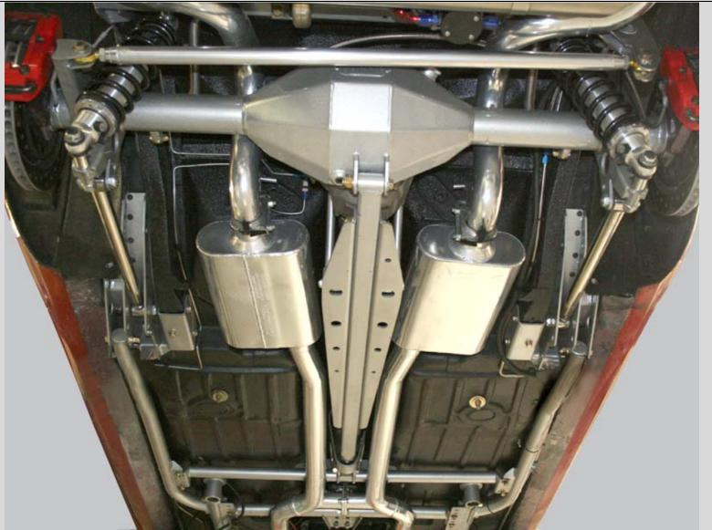
The Torque Arm rear suspension completely installed. The TCI Camaro uses 2<sup>1</sup>/<sub>2</sub> inch exhaust system and Flowmast mufflers. Everything is tucked up close and tight so installing the driveshaft should be done before installing exhaust system and leaving one of the pinion support tubes off until the driveshaft is installed.
