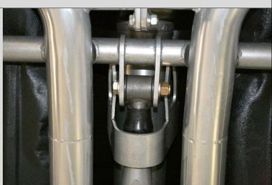
The slider is installed and centered. The Torque Arm cross member has exhaust cut out relief's to allow the exhaust pipes to be tucked up higher for more ground clearance.
