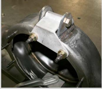
The torque arm tabs are welded on by using the supplied fixture tool. Bolt fixture to the lowest 2 third member bolts flat against the housing flange. Bolt on the two supplied tab using the  $\frac{1}{2}$  by  $\frac{3}{2}$  inch bolt and with the longer tab to the passenger side of the housing. Bottom of tabs may need sanding to fit. Weld outside and wrap welds also to the inside.
